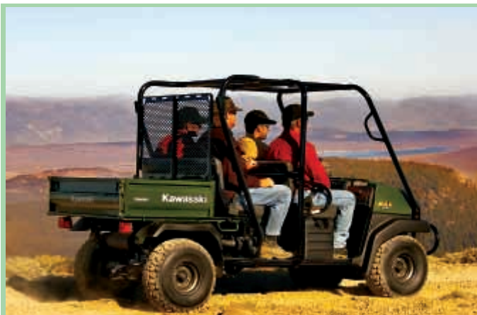
FARM SHOW associate editor Dawn Throener recently traveled to Lincoln, Neb., to test-drive Kawasaki's new “4 to 2” utility vehicle which has a second-row passenger seat. When extra cargo space is needed, it quickly converts to a 2-passenger rig by folding down the back seat. Dawn reports that the new Mule is a powerful machine with a smooth ride. You can check it out at www.kawasaki.com .
