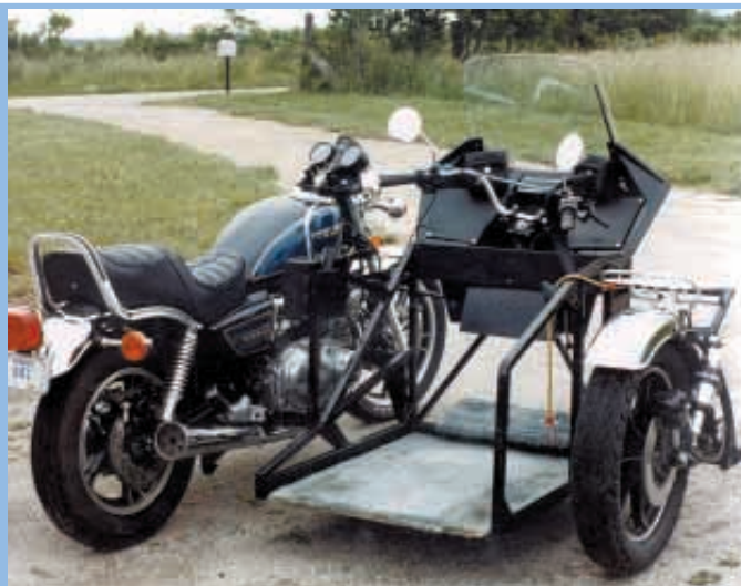
"The idea is to drive the motorcycle while sitting in a wheelchair on the sidecar," says inventor Russell Headley. "If desired, a passenger can ride on the motorcycle."
