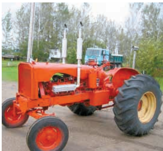
"The results were beyond my greatest hopes," says Clark Carpenter, who repowered his 1955 Allis Chalmers WD 45 with a 283 cu. in. gas engine out of a 1959 Chevy.
