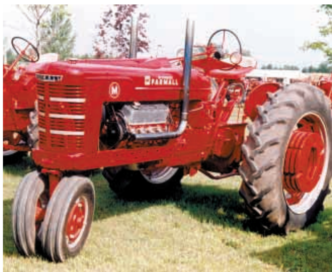
Jim Michealis put a Chevy 454 V-8 engine into this 1950 Farmall M, adding a pair of chrome-plated mufflers. "It makes a nice, smooth-running combination," he says.
