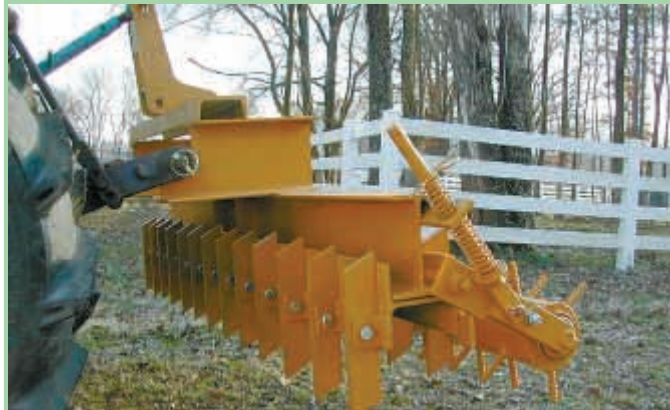
Scarifiers on front bolt to sections of angle iron that are welded to I-beam frame.
