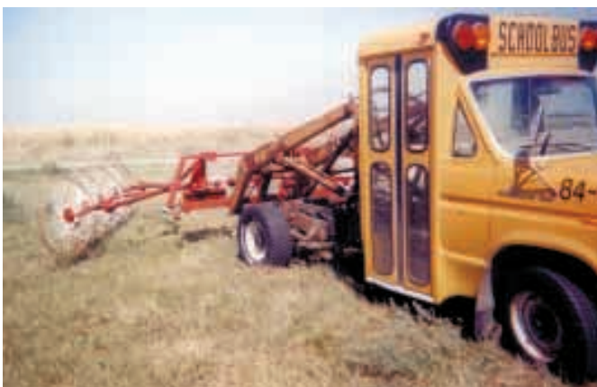
John Maxfield converted a 30-passenger bus into a 10-wheel rake carrier. Front-end loader facing backward on bus frame holds rake.
