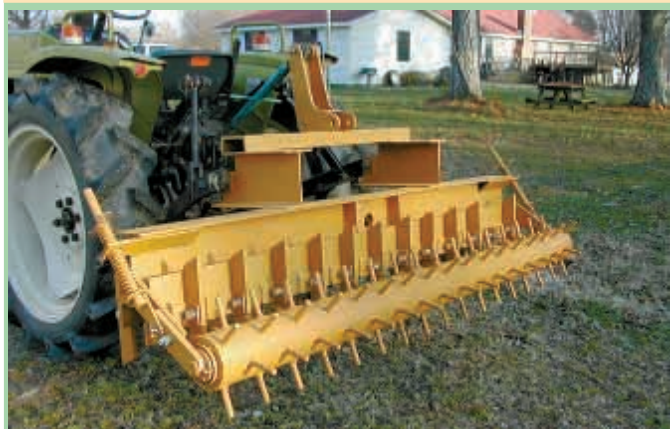
"It does the job of both a tiller and a landscaping box," says Brent Pepper, who built this 5 1/2-ft. wide, 3-pt. mounted landscape pulverizer mostly from scrap metal.
