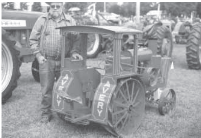
Using photos and specs that he got out of a book, Ed Rupp built this 1/2-scale model of a 1922 Avery 14-28 tractor.
