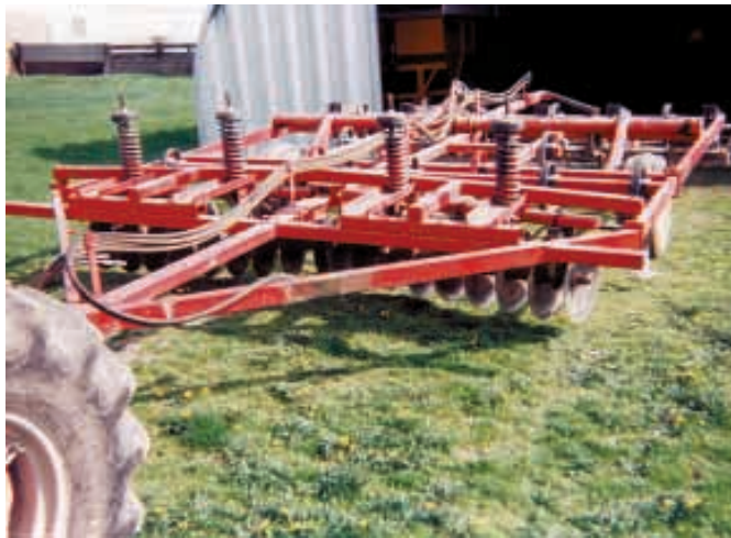
The Weavers started with a Brady field cultivator and lengthened the frame by 4 ft. They added a couple disk gangs on front.
