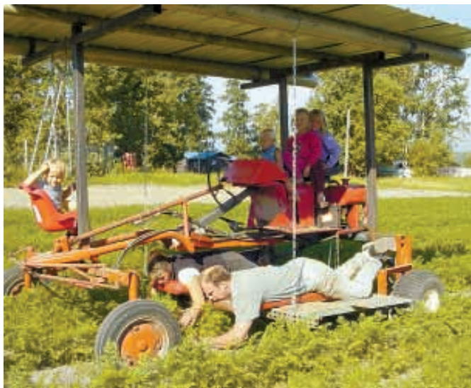
Hydrostatic weeder was made by marrying the back end of a 3-wheel Toro utility tractor to the front end of an Allis Chalmers G tractor. It's controlled by foot pedals so the Herrs can weed their vegetable fields while laying down.
