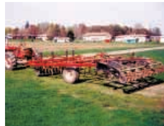
The Weavers started with a Brady field cultivator and lengthened the frame by 4 ft. They added a couple disk gangs on front.
