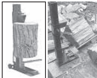
Green's 5-ton manual mini splitter has a foot-powered hydraulic wedge. It splits logs up to 19 in. long.
