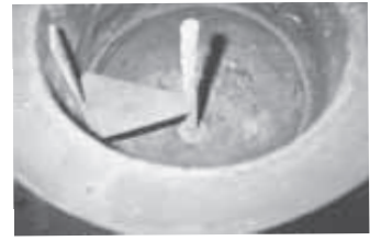
He used steel pipe and plate steel to build the fire pot (left). DC motors power the feed auger as well as a stainless steel agitator inside firepot.
