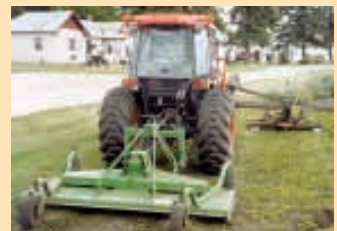
Houska uses same offset mounting bracket on loader to operate a 5-ft. front-mount wide mower.
