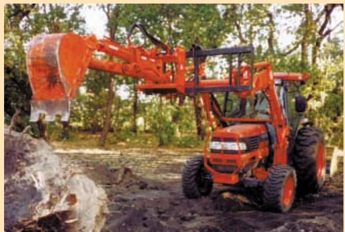
Backhoe boom can be hydraulically shifted from side to side along 6 1/2-ft. wide mounting bracket, which was originally designed for a loader-mounted round bale fork.
