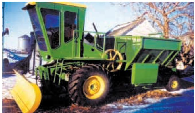
Home-built bale shredder mounts on back of combine frame. Bale arms at rear load bales into hopper.
