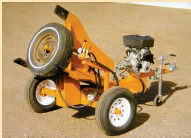
Eugene Luoma's machine is powered by an 18 hp V-twin electric start motor. A single hydraulic cylinder powers the jaws that close around wheel.
