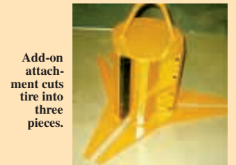
Each crushing arm applies about 50,000 lbs. of force. Cloverleaf-shaped crushed wheel rim comes out of tire easily.
