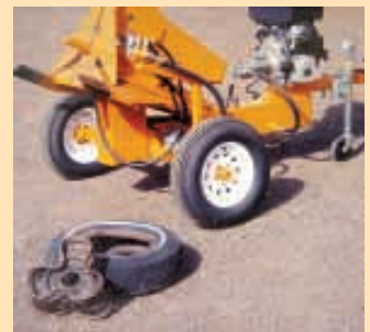
Each crushing arm applies about 50,000 lbs. of force. Cloverleaf-shaped crushed wheel rim comes out of tire easily.
