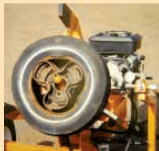
Each crushing arm applies about 50,000 lbs. of force. Cloverleaf-shaped crushed wheel rim comes out of tire easily.
