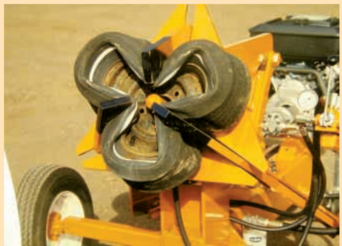
It takes only about 20 sec. total to crush wheel so Luoma says he can squash 120 wheels per hour.
