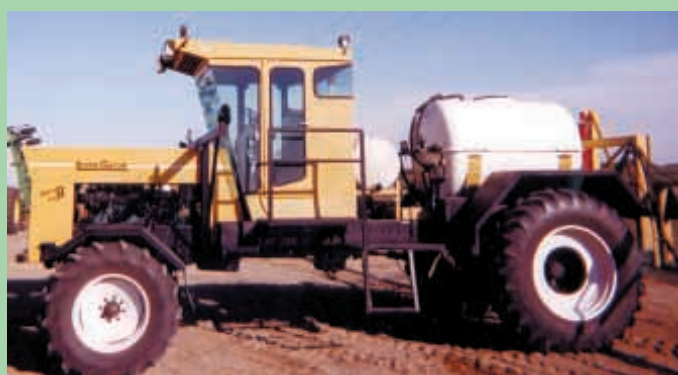
Brian and Tim Levenson converted an old school bus into this state-of-the-art self-propelled sprayer. The cab is off a junked New Holland combine.
