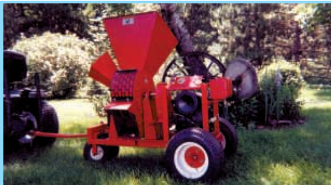
Tad Schreiner's portable wood chipper has two chutes - one on top for leaves and brush and another on front that handles branches up to 3 in. in diameter.
