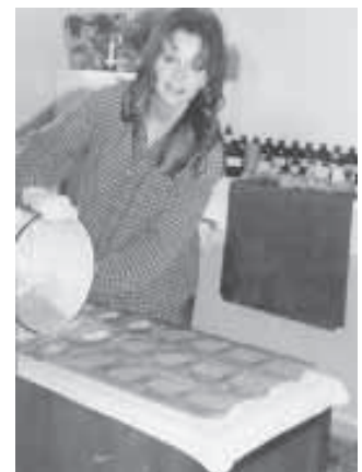
She uses custom-made plastic soap molds. Once the soap has set, she removes bars from their "molds" and "cures" them on shelves for three weeks.
