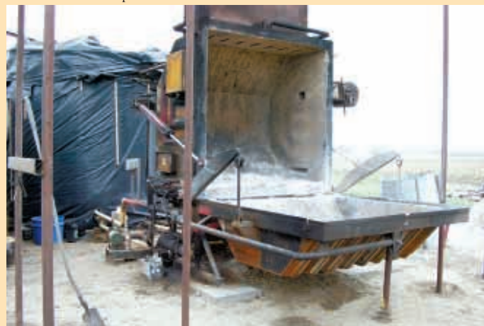
Grate made of 4 chain-driven rollers rotates bale as it burns, improving combustion.
