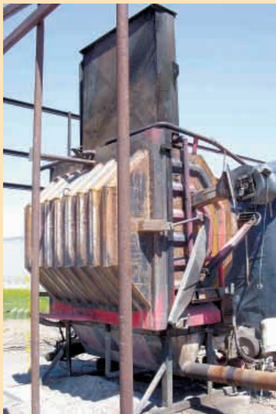
Heatwerks, Inc., makes two models of big bale burners that are being used to heat buildings and dry grain.
