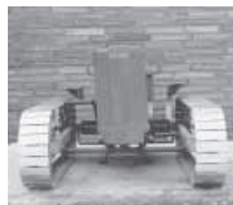
To make the track, Miller mounted no. 40 roller chain around both sets of sprockets, then welded a series of flat steel cleats onto the chain. One cleat is welded onto each chain link.
