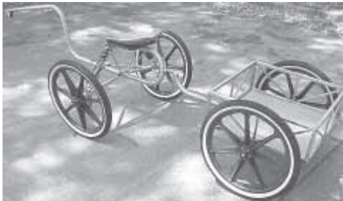
Cart's dorsal hitch extends up and over back of animal to a point just behind the front shoulders, where it attaches to harness.
