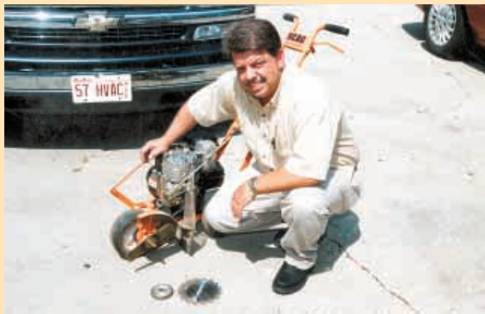
Marty Garrett replaced the edging blade on his lawn edger with a “wobbling” circular saw blade. “It lets me follow along the roots and plane them off at ground level, without tearing up a lot of grass,” he says.
