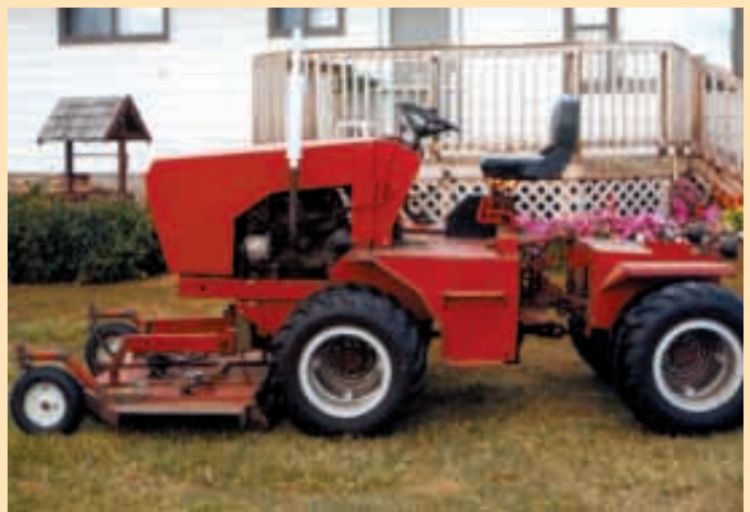
Using mostly junked parts, Harold Tribitt built this 4-WD articulated “mower tractor” equipped with a 6-ft. front-mounted deck that rides on a pair of caster wheels.
