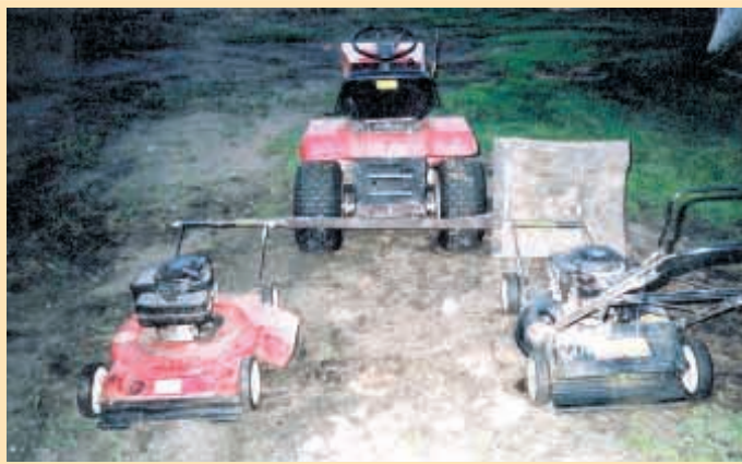
Pulling two 20-in. push mowers behind his riding mower lets Bob Simpson “reduce mowing time in half.”
