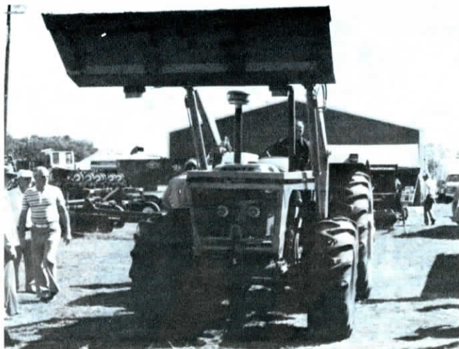
Loader lifts to 17 ft. height and has breaking lift capacity of 5,800 lbs.
