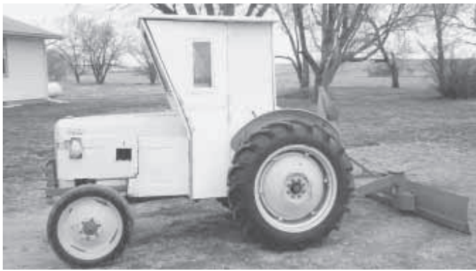
Using 3/4-in. plywood and metal sheeting, Ron Newton made a cab for his Ford 8N.
