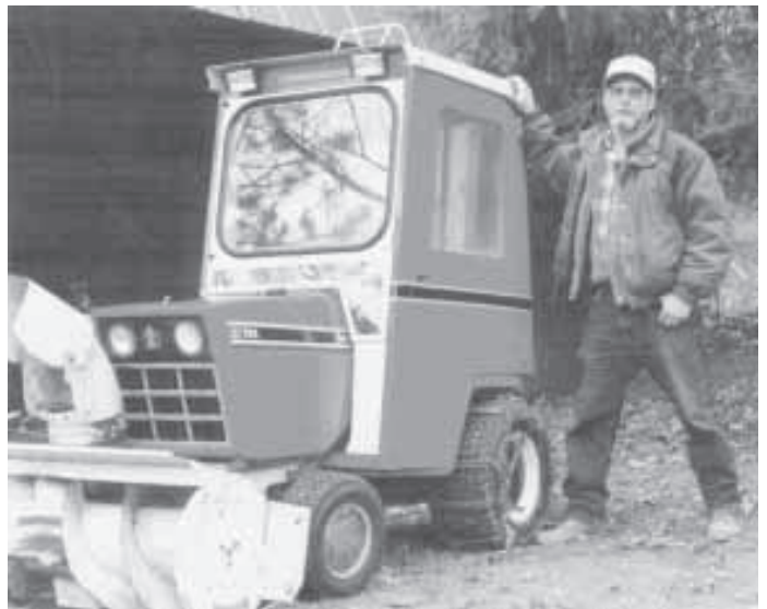
Biech's home-built cab has a hinged glass windshield that lets him easily check engine fluids. Hinge pins pull out so he can remove windshield.
