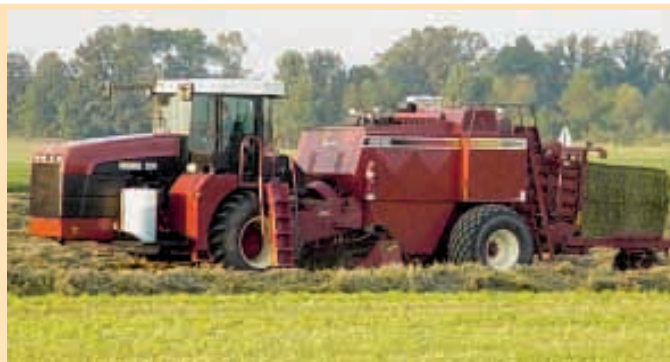
The Fry brothers say advantages of a self-propelled big square baler include: a smoother ride, less maintenance, and shorter turns.
