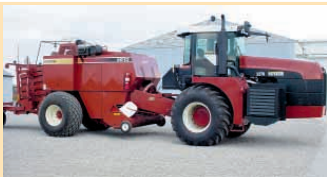
The front half of a Buhler Versatile 2270 4-WD tractor, equipped with a 290 hp Cummins engine, is connected to a Hesston 4910 baler that makes 4 by 4 by 8-ft. bales.
