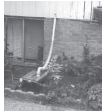
Kirby's passive trap is a box with wire screen on sides (left). He also has a powered trap that uses a vacuum for suction (right).
