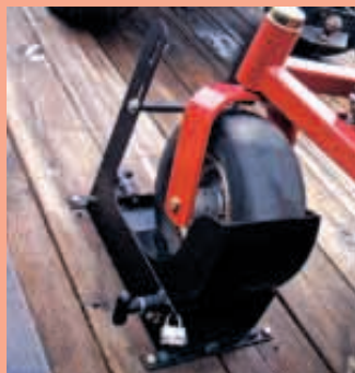
Spring-loaded unit locks onto a single tire.
