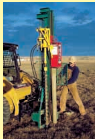
Munro Digger-Driver is equipped with an auger. It lets you drill a pilot hole and then use the driver to pound the post into the hole.
