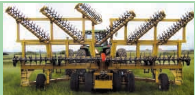
New-style tillage tool consists of a rotating tine-type aerator combined with a Phoenix rotary harrow.
