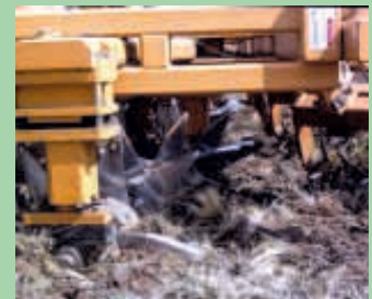
Heavy duty tines fracture the soil up to 8 in. deep with minimum soil disturbance on the surface.
