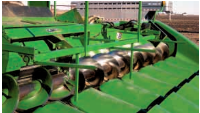
Trash Reel mounts over the center five snouts, keeping material flowing through feederhouse.
