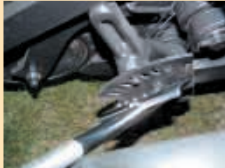
A row of metal ribs on tool release the locking pin on adjusting plate, allowing you to rotate adjusting plate to desired setting.
