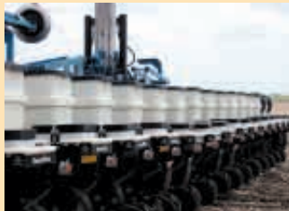
Snap-on box toppers add more than one bushel of capacity to each seed box.
