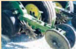
Seed closers bolt onto closing wheel frame and are designed to accept rubber closing wheels. You adjust down pressure by moving a handle.
