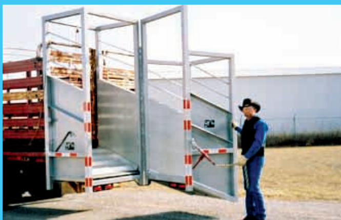
"It lets me use my existing semi livestock trailer to load and unload cattle either from the ground or from a loading dock, eliminating the need for a separate loading chute," says LeRoy Stotts about the conversion chute he built on back of his semi-trailer.
