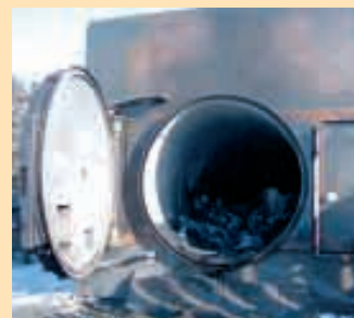
They cut a hole in one end of tank and inserted a 19-ft. long by 7-ft. dia. rail car tank inside. After cutting the end off the 7-ft. tank, they used both tanks' end pieces to make a big double-walled door.
