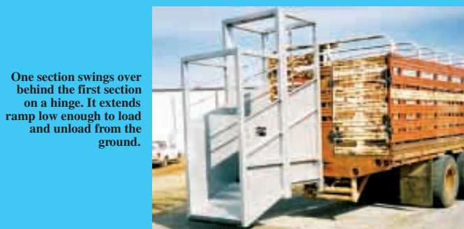
"It lets me use my existing semi livestock trailer to load and unload cattle either from the ground or from a loading dock, eliminating the need for a separate loading chute," says LeRoy Stotts about the conversion chute he built on back of his semi-trailer.
