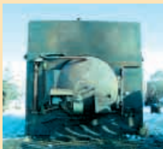
They cut a hole in one end of tank and inserted a 19-ft. long by 7-ft. dia. rail car tank inside. After cutting the end off the 7-ft. tank, they used both tanks' end pieces to make a big double-walled door.
