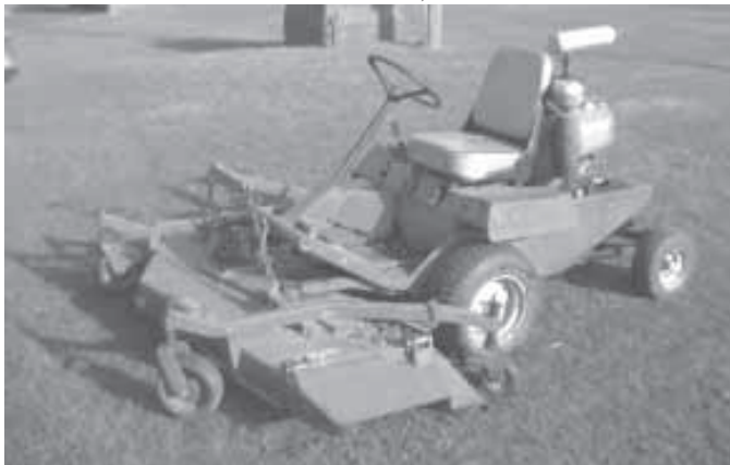
"It has a lot of torque and great traction," says Mike Van Horn about the heavy-duty Toro riding mower he repowered with a big 30-hp Wisconsin engine.
