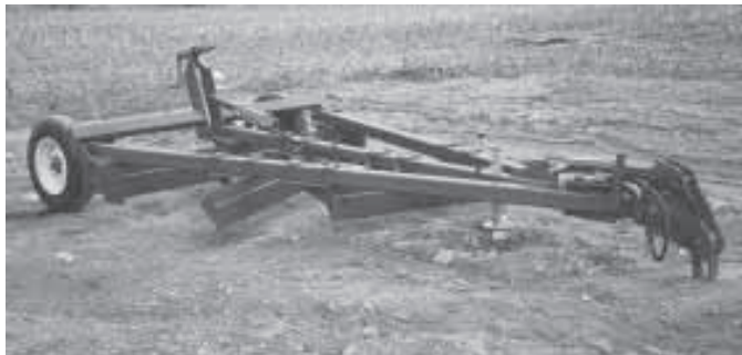
Front and rear cylinders on this 3-blade lane grader allow operator to adjust how aggressive the front blade digs and the rear blade spreads.
