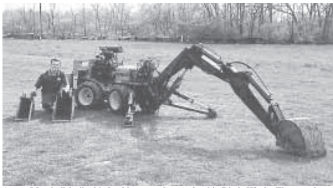
Aaron Marshall built this backhoe attachment for his Ditch Witch. The arm has a stretch of 8 ft. and can dig to a depth of 6 ft.
