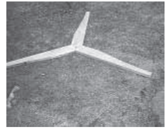
Stan McDonald built a windmill to provide free electricity for a friend. It has 20-ft. long wooden vanes.
