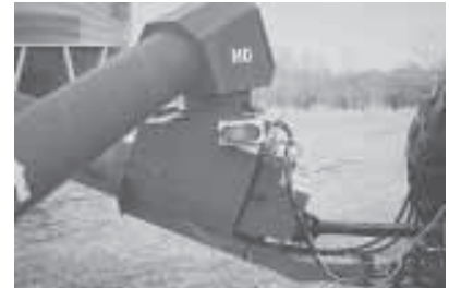
Attached to auger spout, sensor detects when bin is full and electronically signals a magnetic-mount light located on auger tubing.
