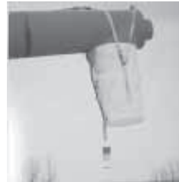
Attached to auger spout, sensor detects when bin is full and electronically signals a magnetic-mount light located on auger tubing.
