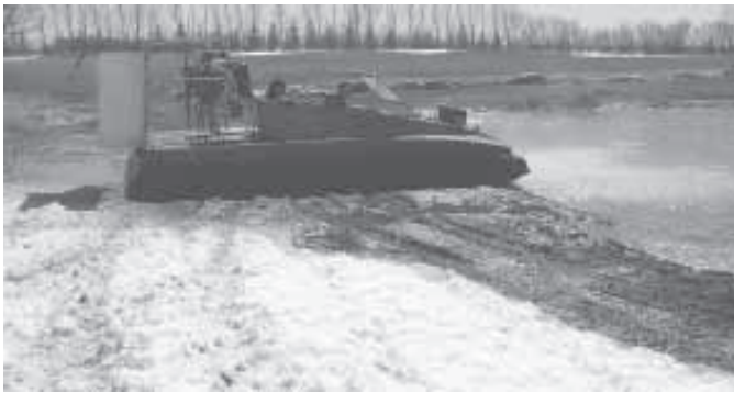
Lightweight hovercraft is made mostly of wood, "and lots of glue," says Kevin Mollenbeck.
