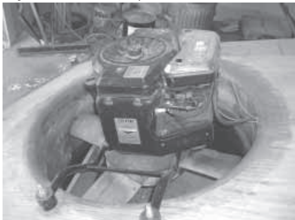
An 18 hp gas engine turns a 34-in. dia., four-blade fan carved from laminated 1 by 6's. Fan pushes air under the hovercraft.
