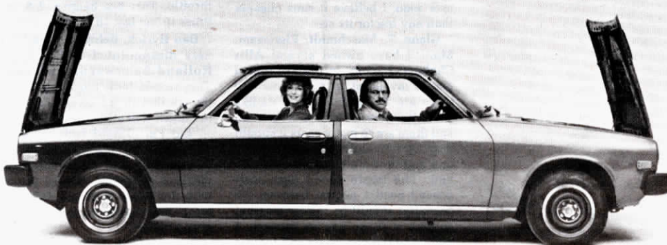
The double car has two engines and steering wheels, and can be driven from either end.
