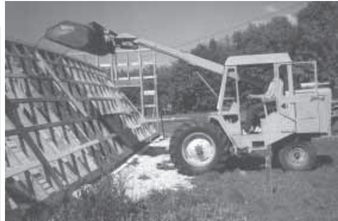
"It makes quick work of jobs around our farm and yard," says Steve Rapko about his home-built telescopic loader boom.
