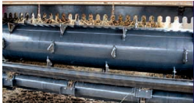
Bale feeding machine's rotor is equipped with welded-on sickle teeth that rotate counterclockwise so material comes over the top.
