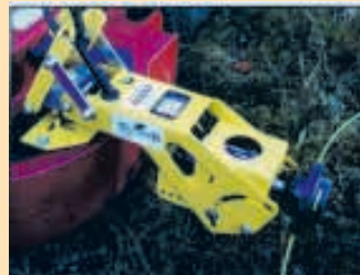
By loosening a wing nut, you can adjust head and use the unit as an edger.
