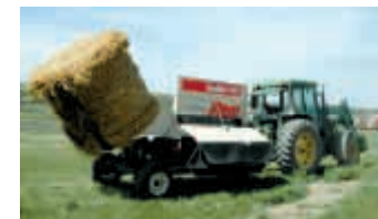
Machine uses sickle knives instead of flails to pull hay off bale and feed it into bunks or windrows.
