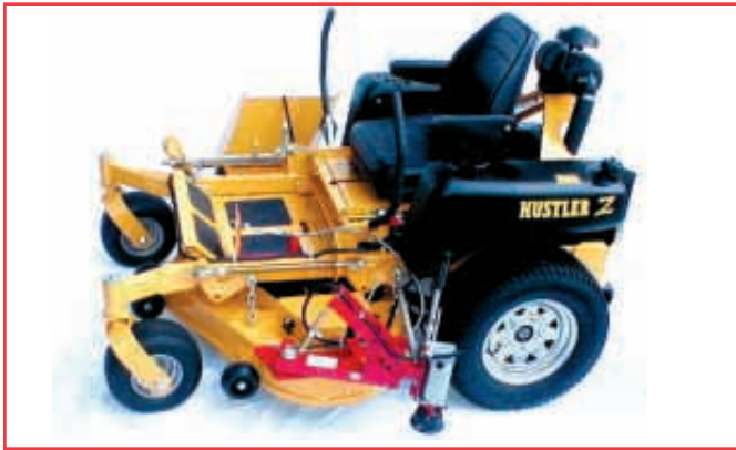
Trimmer mounts on one side of deck and is powered by a self-contained hydraulic pump and motor.
