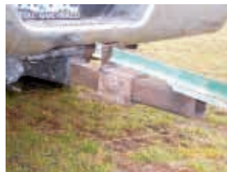
Schulze built this fence post straightener to fit into his pickup's receiver hitch.
