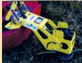
Trimmer can reach out up to 20 in. from edge of mower deck.
