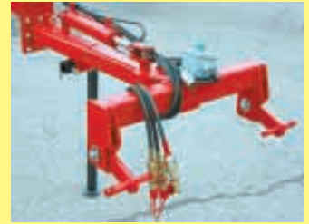
Hydraulic cylinder mounted on tongue extends or contracts as tractor turns.
