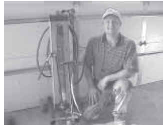
Dean Kolschefske says his transmission flusher requires no electricity and therefore no pumps or motors.
