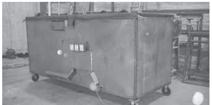
Gerald Bliss built this 10-ft. long "metal cooking" oven that lets him powder coat virtually any kind of metal. It has three heating elements that came out of kitchen ovens.
