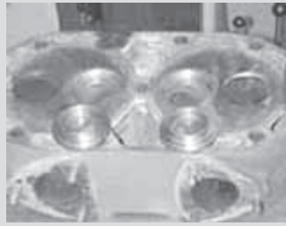
This cylinder head, off a 1915 Titan 1020 tractor, was cracked. Hine custom-machined the head and also made new valve seats for it. Then he pushed the seats in and reground them.
