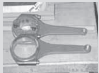
He built this cam drive mechanism to operate the Otto engine's fuel pump. Top piece has a 1-in. drop eccentric drive in it. Bottom piece is the connecting rod.
