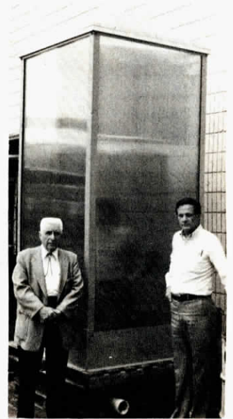
Solar box (5 by 5, by 9 ft. tall) is enclosed on three sides by special material that captures, holds solar heat.
