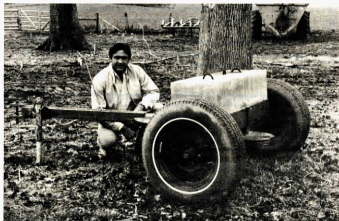
Concrete weight is positioned slightly forward to stabilize front tongue.
