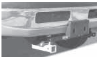
"It lets you move trailers and wagons around in the spring and summer without having to remove the snowplow mounting bracket, which is a big job," says Lee Nemec.
