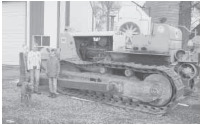
When the engine wore out on his IH crawler, Kevin Cohrs replaced it with the diesel engine out of an IH 4-WD tractor.
