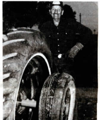
Wire is guided onto an auto wheel mounted on the tractor axle hub.
