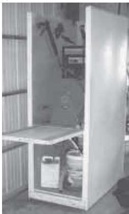
Cabinet mounts on four canister wheels and stands 8 ft. high. Front side of bottom compartment doubles as a folding shelf that folds out at pickup bed height.
