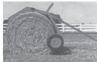
To load, you back up so a short tooth on back slides under bale (top) then pull on a rope which releases claw to drop down over bale (below).
