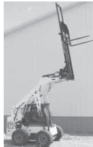
Tele-Fork quick-taches to skid loaders or compact tractors with quick-tach loader systems.
