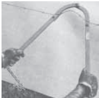
Fixer is spread wide to hook onto wire and then pulled together. A chain holds jaws together while wire is tightened.
