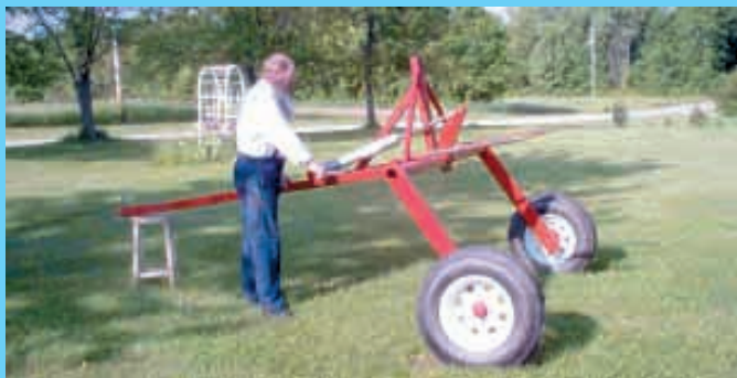
Spears mount on a pivoting mechanism that's raised and lowered by jack.
