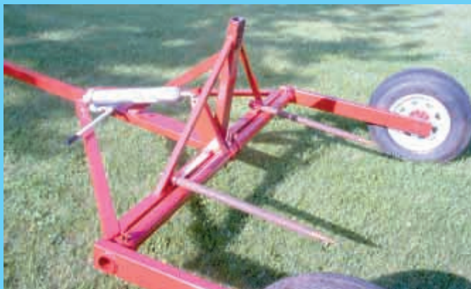
Two-wheeled rig has a ball hitch on front and three bale spears on back.
