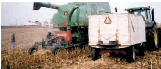
Here a "stover caddy" is pulled behind a Deere 9750 combine. It blows material off to the side into a tractor-pulled wagon.
