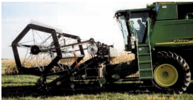
Iowa State University researchers are testing ways to gather crop residue cheap. This Deere 9750 has a giant experimental 8-ft. dia. reel on a 2-tier corn head that collects ears in one stream and stalks in another.
