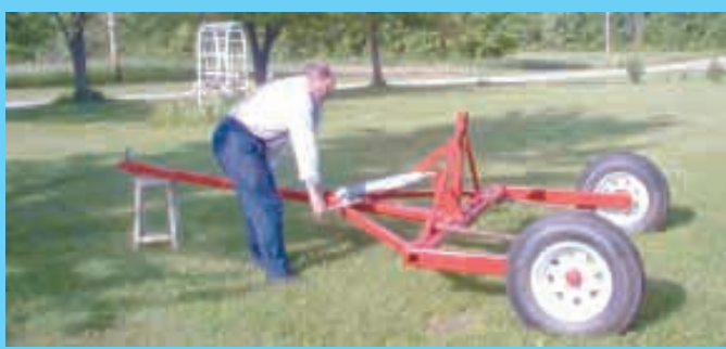
To load a bale you back up and spear bale, then use jack to pivot bale up off the ground.
