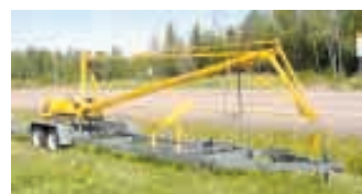
Crane folds down for transport.
