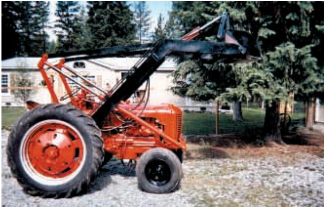
"It gives me full-time hydraulics on an older tractor without having to spend thousands of dollars for a new tractor," says Bill Wilson, about the hydraulic-operated front-end loader he built for his 1949 Case DC tractor.
