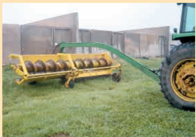
To build auger merger, the Staubers took the 10-ft. hay header off an old Deere 630 self-propelled windrower and lengthened it by 6 ft. They attached it to a Hesston hydraulic haybine frame, using the Hesston hydraulic system to drive the hay head.
