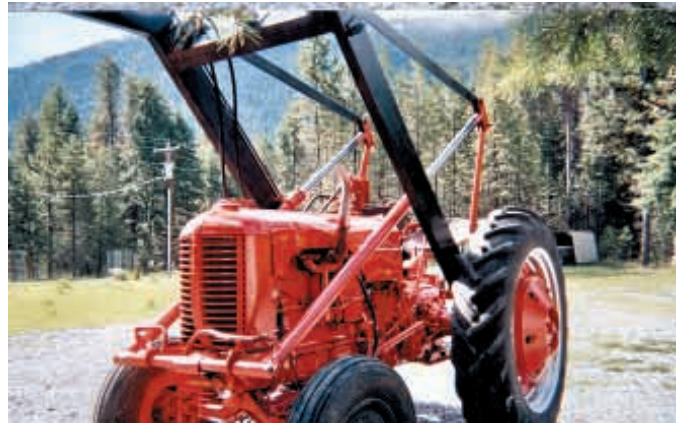
"It gives me full-time hydraulics on an older tractor without having to spend thousands of dollars for a new tractor," says Bill Wilson, about the hydraulic-operated front-end loader he built for his 1949 Case DC tractor.
