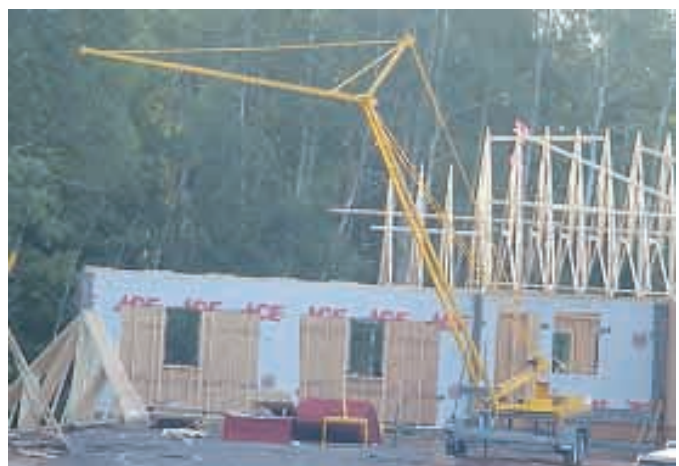
Trailer-mounted crane is designed to be pulled behind any pickup. It's controlled by four 12-volt electric motors that are powered by a pair of deep cell batteries.
