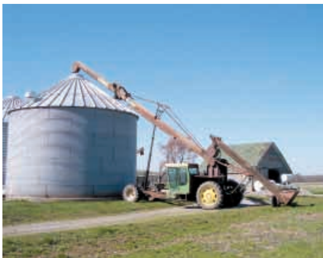
Self-propelled rig is equipped with a 76-ft. long, 14-in. dia. bin auger that can move 800 bu. of grain in 10 minutes. An 18-ft. fill auger mounts on back.
