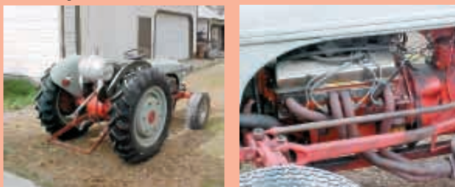
To ready tractor for the Corvette 327 engine, Shafer had to lengthen hood 1 1/2 in.
