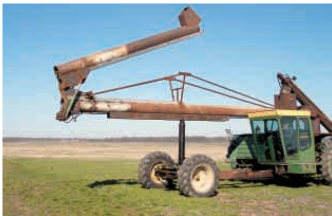
A 22-ft. section at end of 76-ft. auger folds back on top of main auger when in transit.
