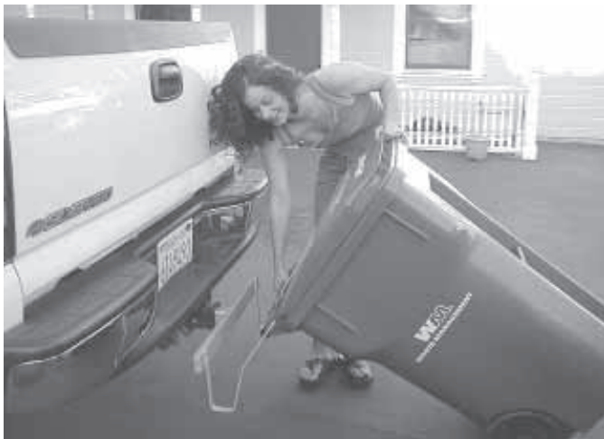
Trash Caddy can pull two big 64-gal. trash containers at once behind vehicle. To use it you tilt container down and hook handles onto a pair of prongs.
