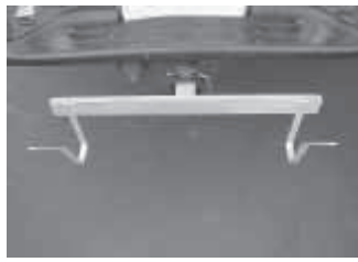
A 28-in. wide steel bar with two hooks attaches to receiver hitch.
