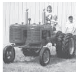
Bill Bradley and son Mark built "twinned" Farmall tractor by joining a 1947 BN with a 1941 A.
