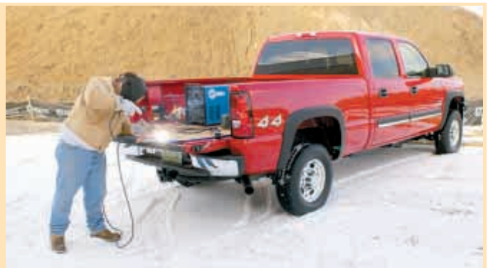
Built-in AC power system works directly off pto gear found on transmissions of many newer pickups.
