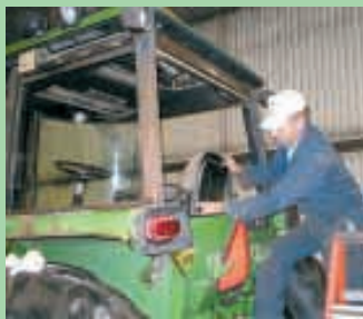
Each cab is given a general rebuild, with new fenders, doors, upholstery, glass, etc.
