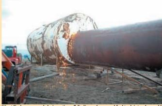
Giant firebox was made by inserting a 7-ft. dia. underground fuel tank into a larger 11-ft. dia. tank.
