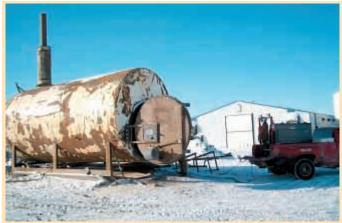
Large capacity bale furnace heats 40,000 sq. ft. at a fraction of the price of LP gas.
