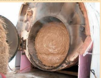
Up to three 5 by 6-ft, round bales can be loaded into furnace at one time.
