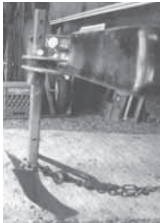
Digger consists of a shovel with a metal bracket on shank that bolts to pickup bumper. A length of chain from pickup frame down to shovel provides additional support.
