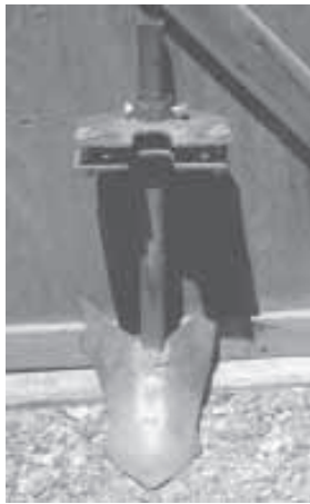
Digger consists of a shovel with a metal bracket on shank that bolts to pickup bumper. A length of chain from pickup frame down to shovel provides additional support.
