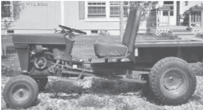
Bill Wilson built his own Gator-type utility vehicle by stretching out a 1971 Minneapolis Moline garden tractor, fitting it with a bus seat, and mounting a cargo box on back.
