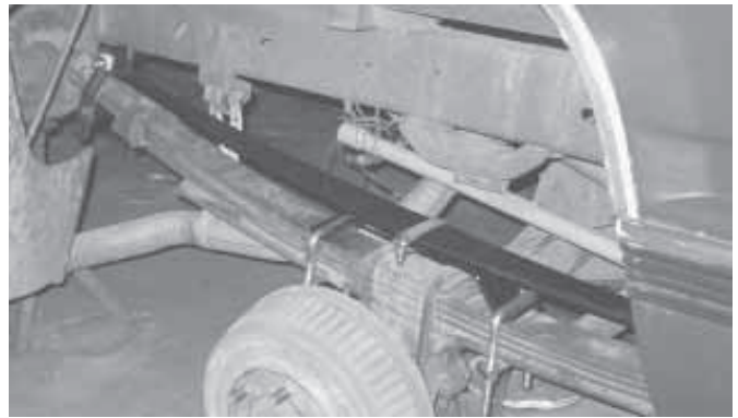
"SuperSprings" are single leaf springs that attach to the original spring, with rolling shackles at each end that self-adjust to movement of existing spring, says Mr. Truck, AKA H. Kent Sundling.
