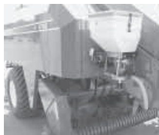
Granular applicators mount directly on hay and silage harvesters as well as balers.
