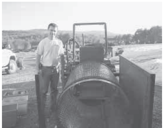
"It's designed to work on pumpkins 8 to 12 in. in diameter," says Mike Clark about his small-scale pumpkin "de-seeder."
