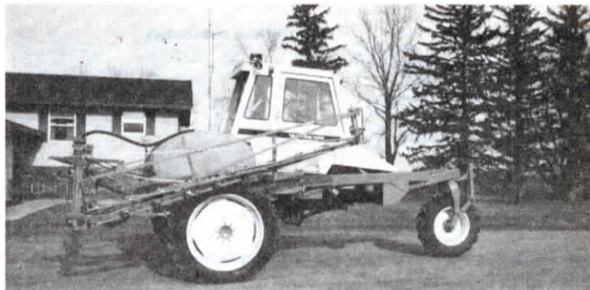
Sprayer boom raises and lowers hydraulically from 15 to 40 in. high.
