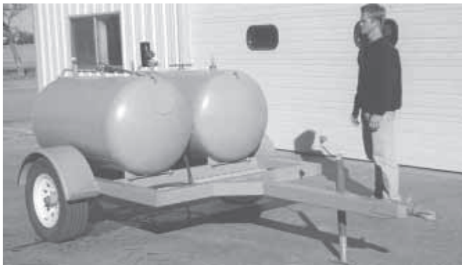
"I spent about $300 to build it. A comparable commercial unit would sell for up to $8,000," says Lonnie Nichols about the portable "oil vac" he built out of an old propane tank.
