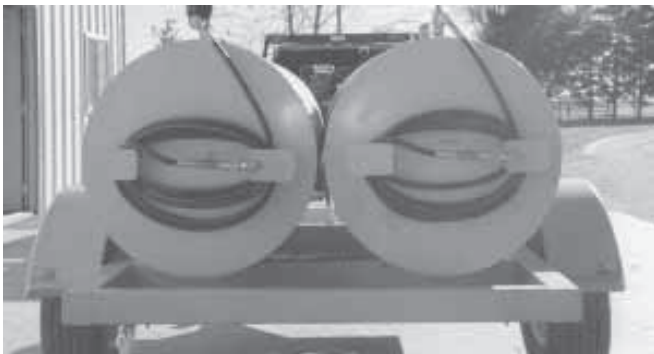
Trailer-mounted rig has twin 200-gal. tanks.
