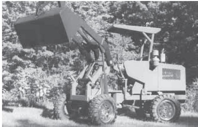
**Mark Adams used two 1986 Suzuki Samurai rear-ends to make this 4-WD, articulated skid steer loader. It's powered by a 4-cyl. Wisconsin engine.**
