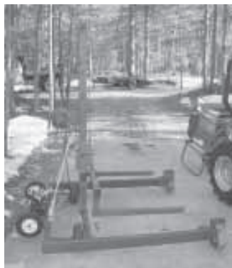
Hoist is equipped with a 12-volt, battery-powered winch that makes it easy to lift heavy items.
