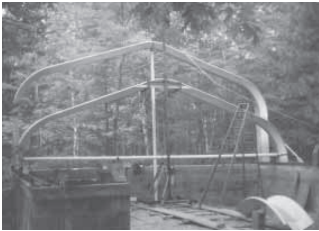
Pehovic has used his home-built "column hoist" to do everything from putting up buildings to drilling a well.
