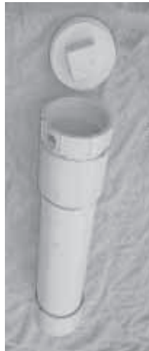
Thick-walled PVC pipe is used to make a cheap safe.
