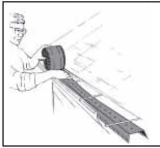
Plastic cover stops leaves from clogging gutter; leaves dry up and then blow away.
