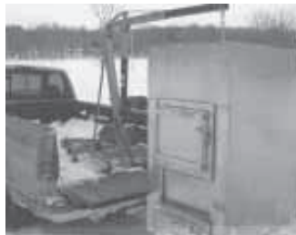
Middleton regularly lifts 600-lb. furnaces, but he thinks it would lift 1,100 lbs.
