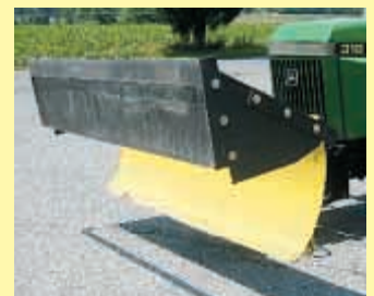
Scoop opens up to dump material where needed. It can be removed with four bolts.
