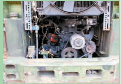
Abandoned Owatonna skid steer and junked Toyota Corolla were combined to make a $650 skid steer loader. Its first job was to pick up what was left of the Corolla and haul it away.
