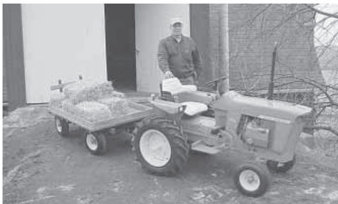
After making cardboard mock-ups and 500 hours of labor, Weisbrod ended up with a half-size replica of the classic Deere tractor.
