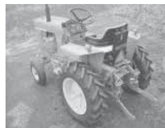
Wheels, hitch, brakes and pto were used from the original JD 318 garden tractor.
