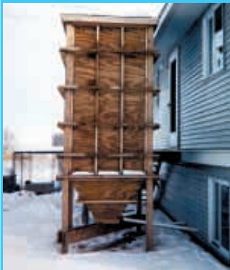
Corn moves about 30 ft. from outside bin to shop vac, which hangs above corn furnace. Corn simply drops out of shop vac into furnace hopper.
