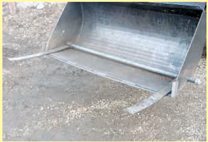
“The fork leaf springs and pipe make a cheap, easy add-on to any bucket,” says Fred.
